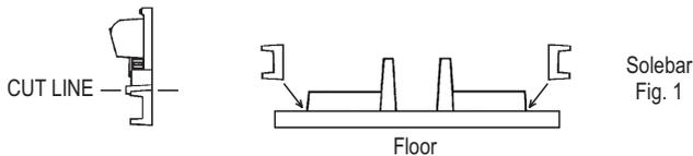
Carefully file the ends of the sides so that they are square and a good fit with the wagon end. Glue the sides to the ends to form an open box. Note that the sides fit between the ends. Ensure that the louvres on the sides and ends are flush and the corners are square before putting the assembly aside to dry.
